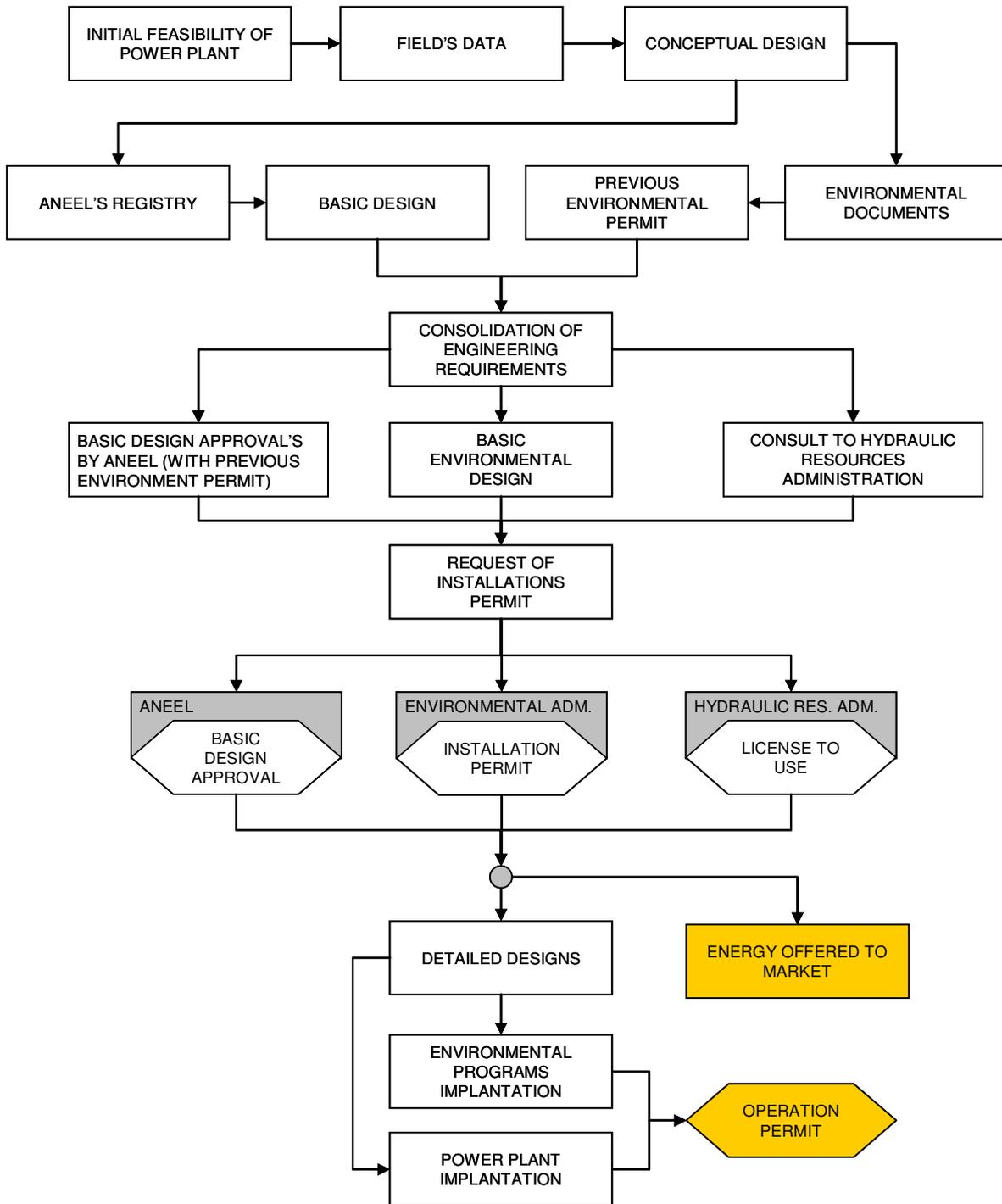
Fig. 2. process to develop and construct a Small Hydroelectric Power Plant (SHPP).
